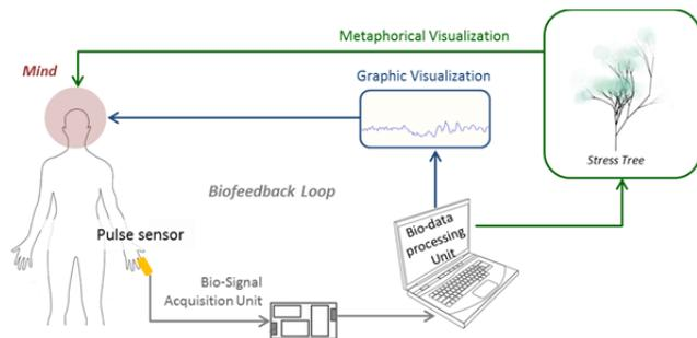
**Figure 4. The framework of HRV biofeedback system**
